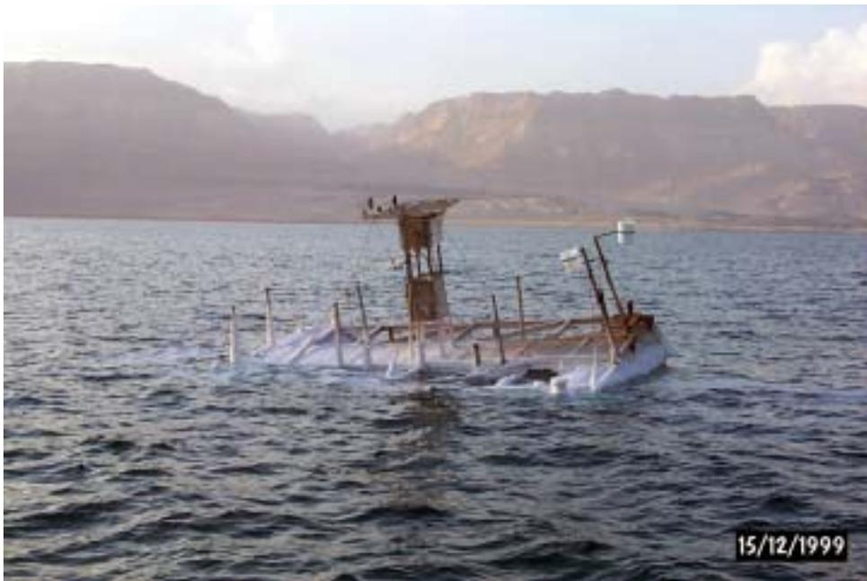
**Figure 3.** Meteorological buoy covered with salt and on the verge of sinking.
